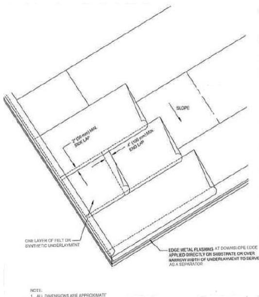
Figure 10-16 Underlayment over Rigid Insulation
