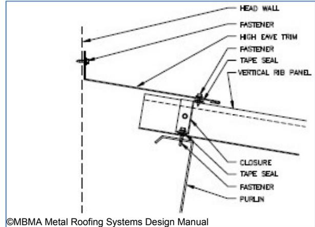
©MBMA Metal Roofing Systems Design Manual
